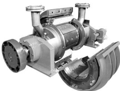
Fig. 4.31 The cylindrical refiner Papillon™ (Andritz), with an open housing for plate change.
