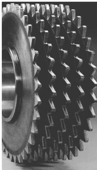
Fig 3.23 Dentated discs in a RaisedRollDisc Thickness Screen [40].
