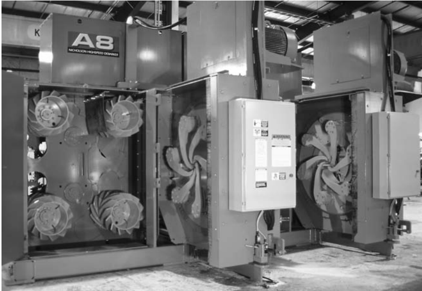
Fig. 3.8 Nicholson A8 Debarker with tandem debarking rings [15].
