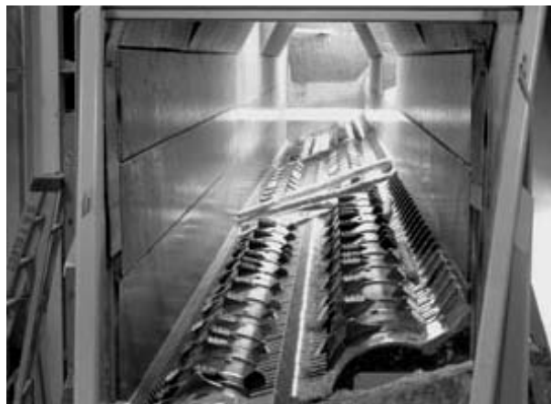
Fig. 3.5 Rotary debarker: the rotating plates spin the logs in the casing [14].
