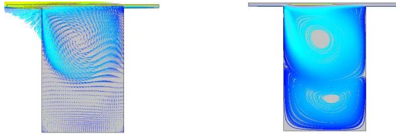
Figure 30: Vector plot (left) and streamline plot (right) at midplane (62.5mm) in the stator.
