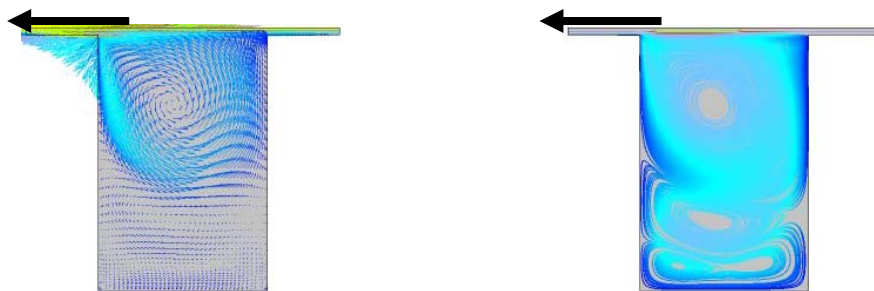
Figure 29: Vector plot (left) and streamline plot (right) at midplane (62.5mm) in the rotor
